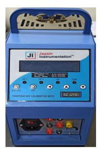
**Purpose:** "Ji" Temperature Calibration bath is used to obtain precise temperature for calibration of Thermocouples & PRTs, SPRTs.
