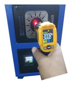
**Purpose:** "Ji" Black body source calibrator is used to calibrate infrared thermometers with precision.
